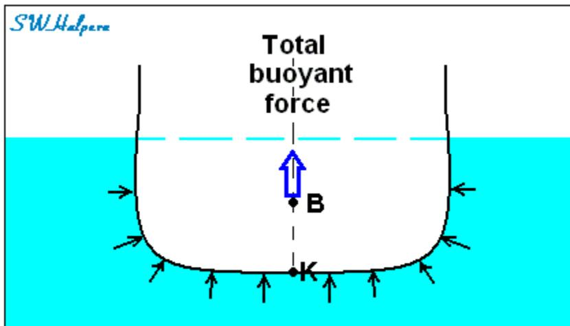
When a ship is at rest on an even keel in calm water, the forces of buoyancy (B) and gravity (G) are equal and opposite, and lie in the same vertical line, as shown in the figure below.
