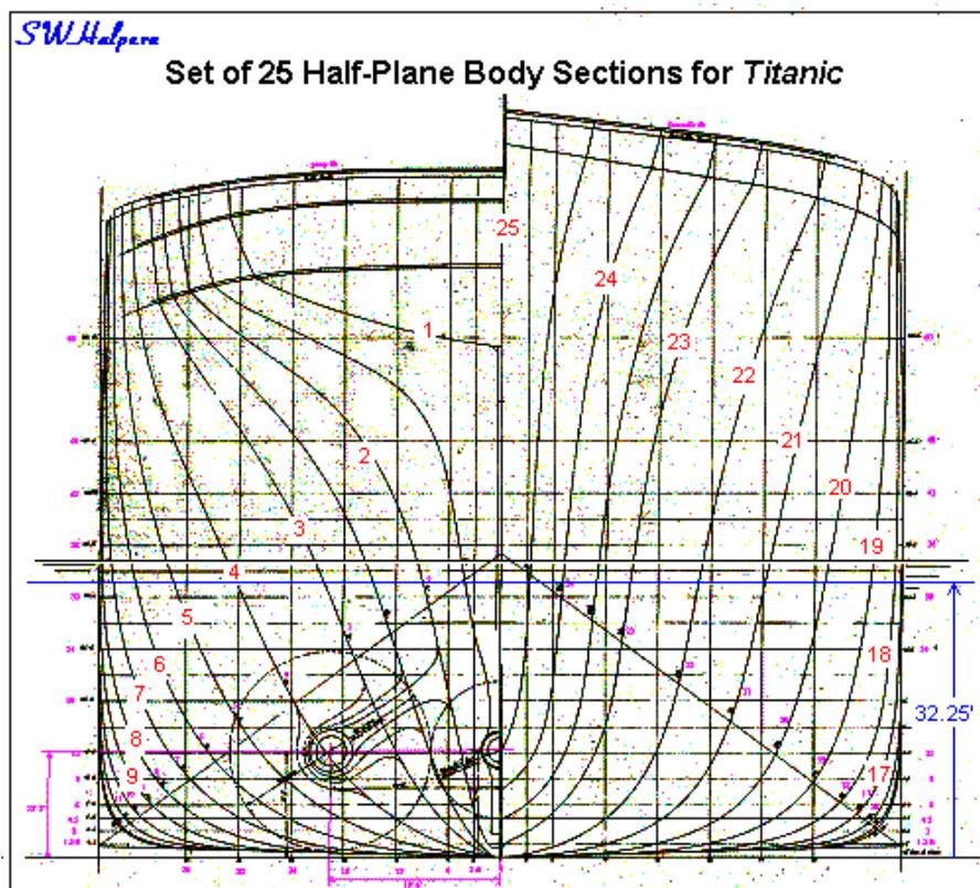
Using  $N = 25$  equally spaced half-plane sections, we can apply Simpson's first rule for integration to determine the waterplane area at a height of 32 ft 3 in above the keel. The rule formula using half-plane sections is:
