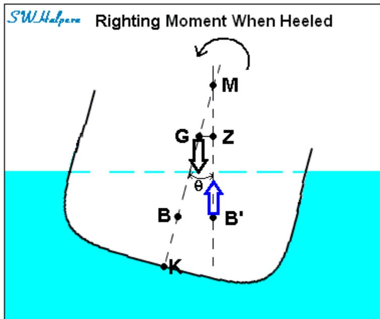
The righting moment is usually taken about the center of gravity point. It is the product of the force of buoyancy times the distance GZ that separates the line of action of the buoyancy force from the center of gravity as shown. The distance GZ is called the “righting arm.” Since the force of buoyancy must equal the weight of the ship, the restoring moment is simply equal to the ship’s displacement in tons times the length of the righting arm in feet. The result will be in foot-tons.
