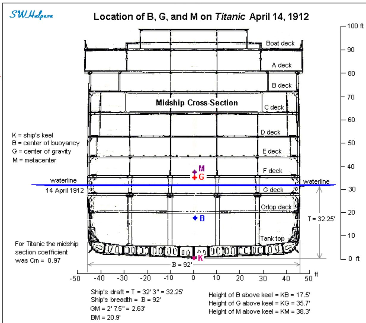
It should also be mentioned that Harland & Wolf naval architects had once calculated the location of the center of buoyancy in the fore-aft direction for *Olympic* assuming a displacement of 51,290 tons at a draft of 34 ft. 3 in. for the ship on an even keel. They found the center of buoyancy to be located 5.7 feet *aft* of amidships. The center of gravity, of course, would be directly above the center of buoyancy in that condition. In doing this they used a set of Bonjean curves.<sup>7</sup>
