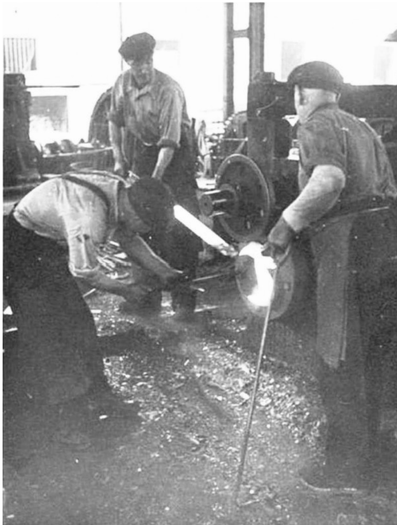
(5) One of the 'Hingley' mandrels at work on small scale chains (Jonathan Smith Collection)
