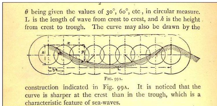
**Figure 2: Trochoidal waves in Theoretical Naval Architecture**
